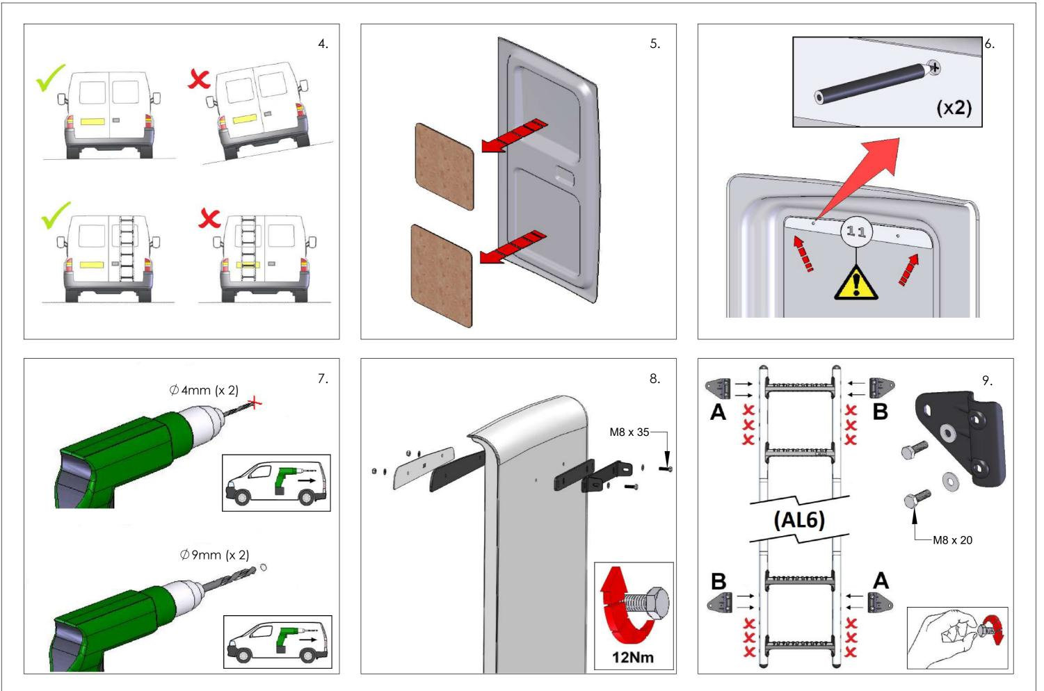
LK33\_b Aluminium Ladder Fitting Kit, T5 & T6 Low Roof (4 Of 5)
